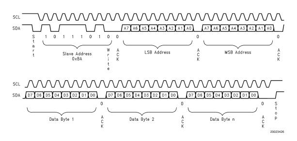
FIGURE 19. I<sup>2</sup>C Compatible Write Sequence
