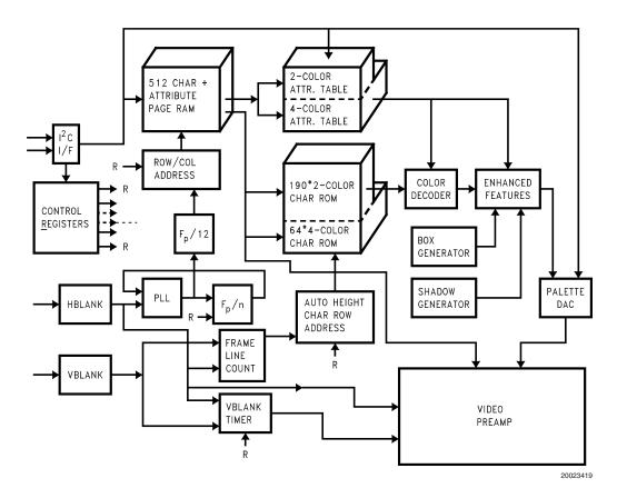
FIGURE 12. Block Diagram of the OSD Generator
