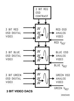
FIGURE 13. Block Diagram of OSD DACs
