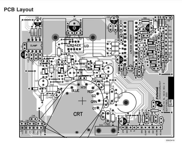
FIGURE 11. LM123x-LM246x Demo Board Layout
