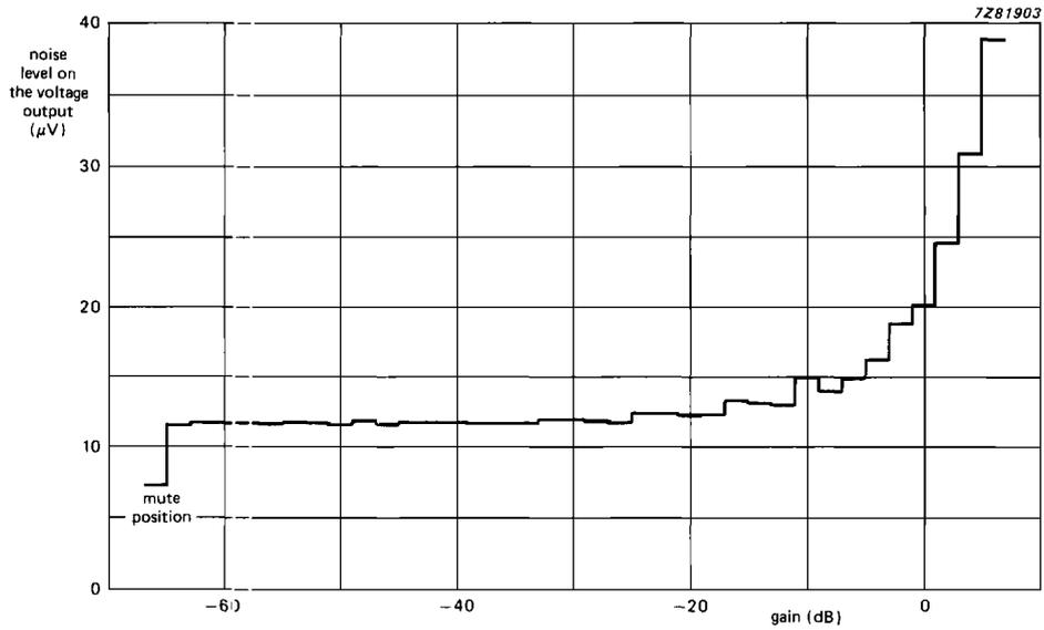
Fig. 16 Noise output voltage as a function of gain; weighted CCIR468 quasi peak gain, +6 dB to -64 dB;  $V_i = 0\text{ V}$ ,  $R_S = 0\ \Omega$ ;  $R_L = 10\text{ k}\Omega$ ; bass/treble = 0 dB;  $V_{CC} = 12\text{ V}$ .
