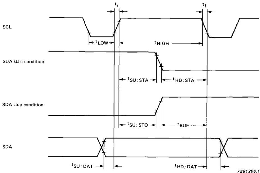
$t_{SU; STA}$  = start code set-up time.
