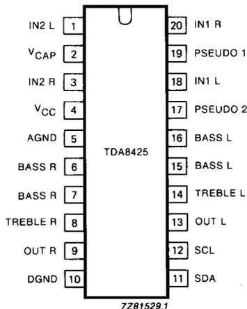
Fig. 2 Pinning diagram.
