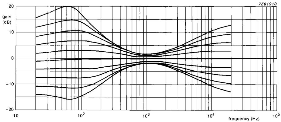
Fig. 17 Frequency response of bass and treble control; bass and treble gain settings = -12 to +15 dB; gain is 0 dB;  $V_i = 0.1\text{ V}$ ;  $R_{Sg} = 600\ \Omega$ ;  $R_L = 10\text{ k}\Omega$ ;  $V_{CC} = 12\text{ V}$ .
