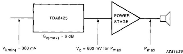
Fig. 24 Level diagram.
