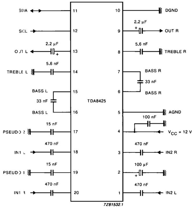
Fig. 25 Test and application circuit diagram.
