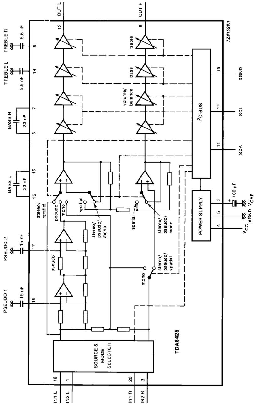
Fig. 1 Block diagram.
