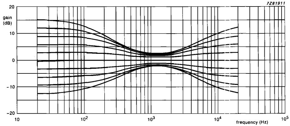
Fig. 18 Tone control with T-filter.
