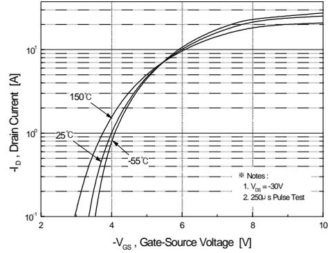
**Figure 2. Transfer Characteristics**
