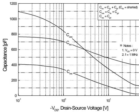
**Figure 5. Capacitance Characteristics**
