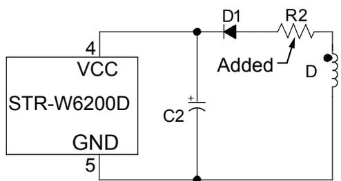
Figure 6. VCC pin peripheral circuit with R2
