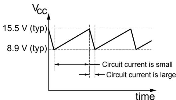
Figure 15. VCC pin voltage at fault latch
