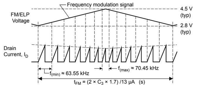
Figure 10. FM/ELP pin voltage and frequency modulation period
