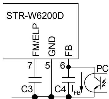
Figure 16. FB pin and FM/ELP pin peripheral circuit
