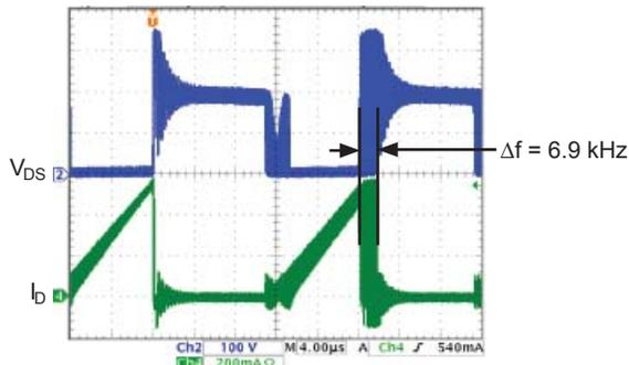
Figure 9.  $V_{DS}$  and  $I_D$  waveforms in frequency modulation
