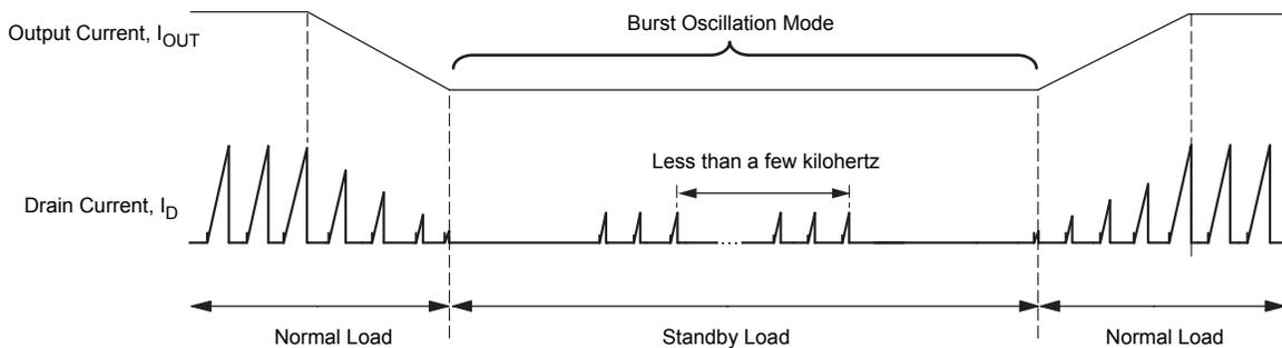
Figure 11. Automatic-Standby mode operation
