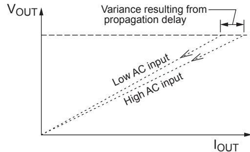
Figure 18. Output current at OCP without input compensation
