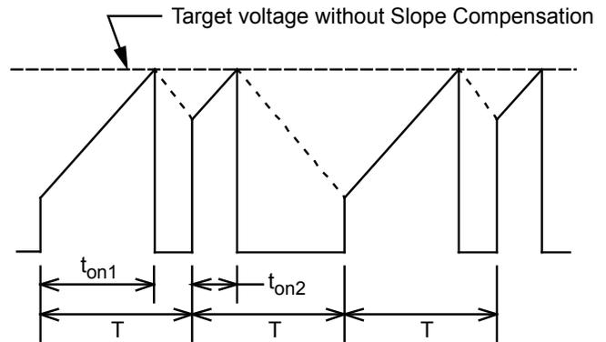
Figure 14. Drain current,  $I_D$ , waveform in subharmonic oscillation
