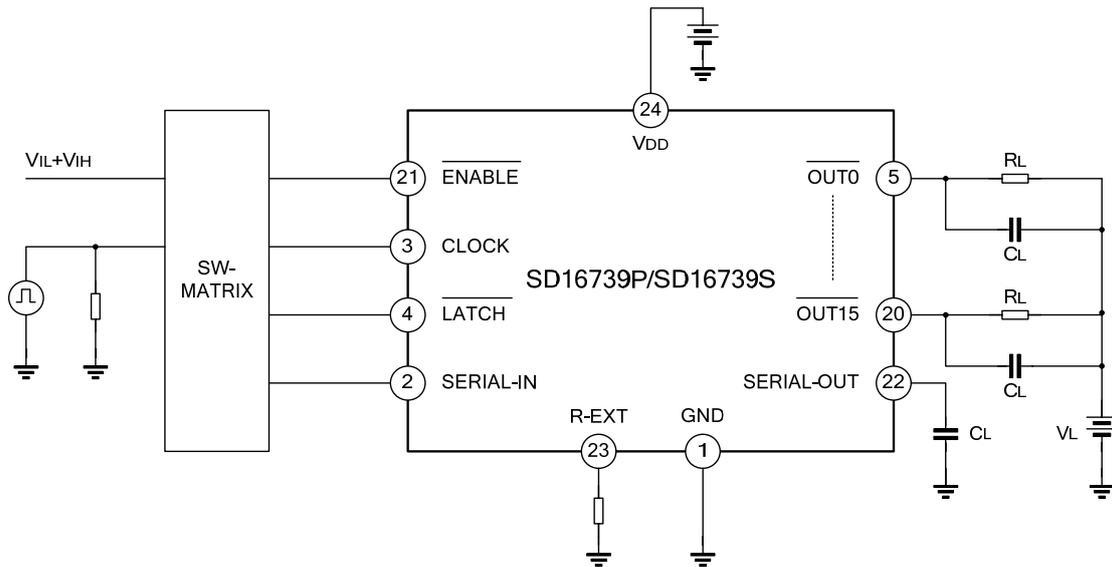
For this test circuit,  $T_{opr}=25^{\circ}\text{C}$ ,  $V_{DD}=V_{IH}=3.3\text{V}/5\text{V}$ ,  $V_{IL}=0\text{V}$ ,  $R_{EXT}=910\Omega$ ,  $V_L=5.0\text{V}$ ,  $R_L=200\Omega$ ,  $C_L=10\text{pF}$ .
