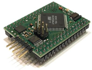
**Connector Kit** – Crumb128-CAN is being shipped without pin headers mounted, since everybody has it's own favorites (pins male/female facing up/down or 90° angled, etc.). A set of high quality pin headers and receptacles are available as a Crumb128-CAN Connector Kit (see picture).
