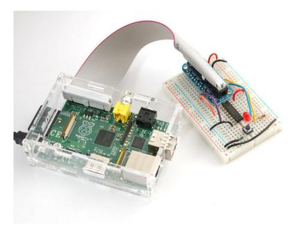
Now that you've finally got your hands on a Raspberry Pi® (http://adafru.it/aHx), you're probably itching to make some fun embedded computer projects with it. What you need is an add on prototyping Pi Cobbler from Adafruit, which can break out all those tasty power, GPlO, I2C and SPI pins from the 26 pin header onto a solderless breadboard. This mini kit will make "cobbling together" prototypes with the Pi super easy.
