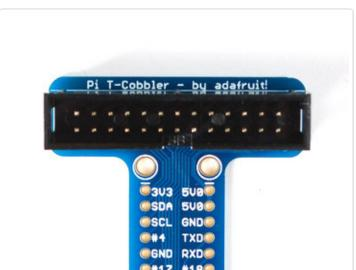
Start by putting the PCB in front of you with the text as shown on the left. Then place the header on top.
