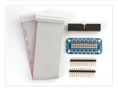
First up, open up your kit and verify you have the components - gray cable, blue PCB, black connector and a stick of male header. The header is breakaway, so it might be one long piece instead of two shorter
