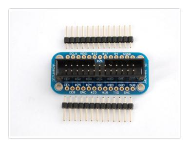
Next break the long piece of header into two 13 pin pieces. You can do this with diagonal cutters, pliers or your fingers
