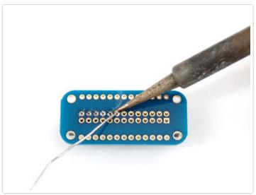
With your soldering iron heated up to 700 degrees F, and some solder, heat up each ring/pin pair for 2 seconds, then poke the end of the solder in to melt it in and make a strong electrical and mechanical connection. Then pull the solder away. Finally remove the iron.
