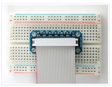
That's it! Now you can turn off the soldering iron and plug the IDC cable. Note that one wire of the cable has a red stripe. That's pin #1. Because the cobbler connector has that notch, you can only put it in the right way (whew!)
