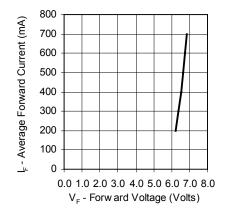
Figure 3. Forward Current vs. Forward Voltage.
