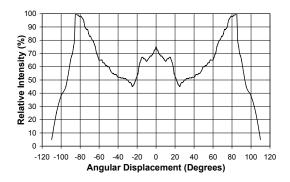
Figure 7. Representative Typical Spatial Radiation Pattern for Luxeon V Star.
