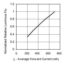
Figure 4. Relative Luminous Flux vs. Forward Current at  $T_J = 25^{\circ}C$  maintained.
