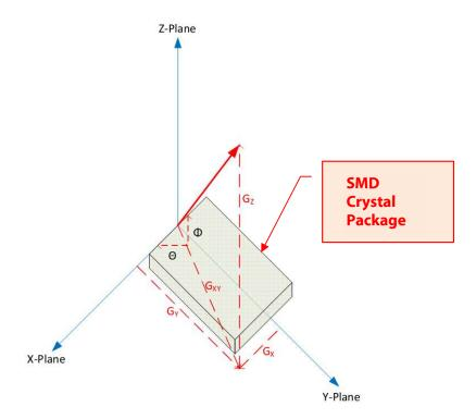
Figure 4: Magnitude of Acceleration Relative to Crystal Package
