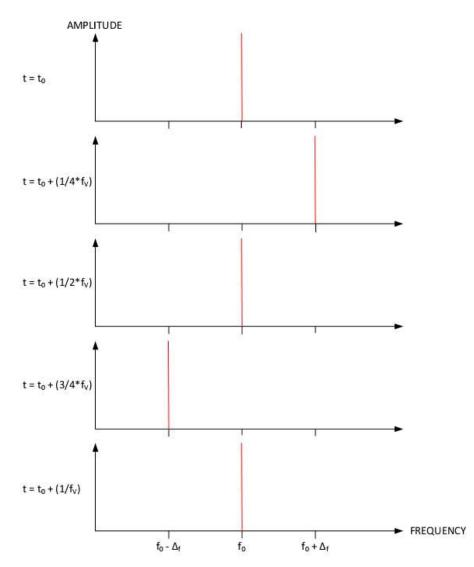
Figure 2: Instantaneous Frequency during one Vibration Cycle
