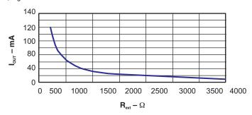
Figure 12. I<sub>OUT,target</sub> vs R<sub>ext</sub>
