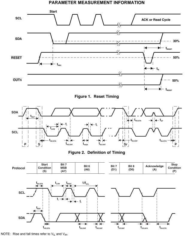
Figure 3. I<sup>2</sup>C Bus Timing
