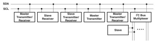
Figure 18. System Configuration
