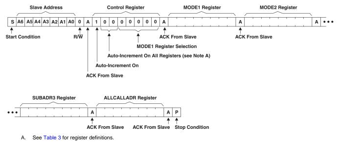
Figure 21. Write to All Registers Using Auto-Increment
