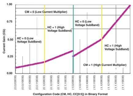
Figure 14. Current Gain vs Configuration Code
