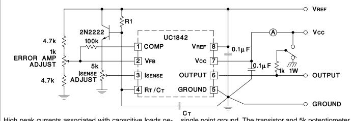
High peak currents associated with capacitive loads necessitate careful grounding techniques. Timing and bypass capacitors should be connected close to pin 5 in a single point ground. The transistor and 5k potentiometer are used to sample the oscillator waveform and apply an adjustable ramp to pin 3.
