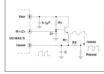
A fraction of the oscillator ramp can be resistively summed with the current sense signal to provide slope compensation for converters requiring duty cycles over 50%.
