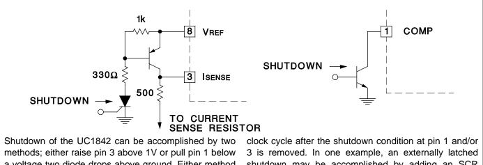
a voltage two diode drops above ground. Either method causes the output of the PWM comparator to be high (refer to block diagram). The PWM latch is reset dominant so that the output will remain low until the next shutdown may be accomplished by adding an SCR which will be reset by cycling VCC below the lower UVLO threshold. At this point the reference turns off, allowing the SCR to reset.
