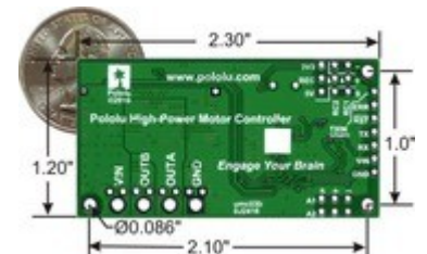
Simple High-Power Motor Controller 18v25 or 24v23 bottom view with dimensions.
