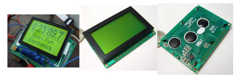
**Description:** This is a framed graphical LCD 64x128 with LED backlight. This unit is a very clear STN type LCD with a simple command interface. This new module includes the negative voltage circuitry on board!
