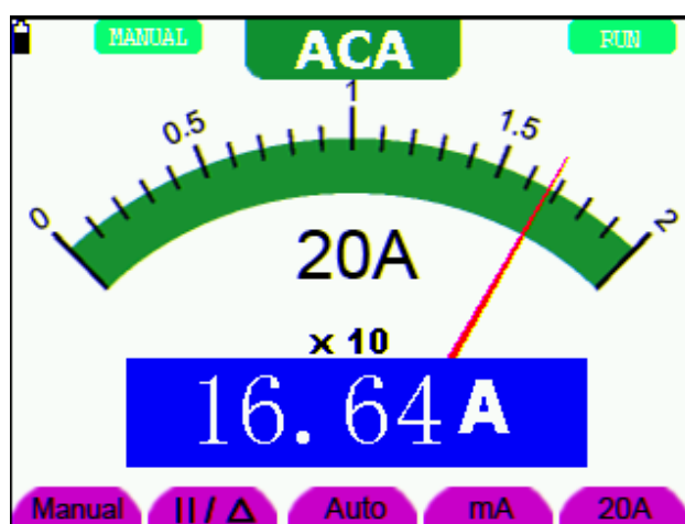
figure 27: AC Current Measurement for 20A
