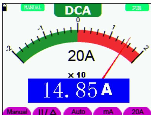
figure 25: DC Current Measurement for 20A
