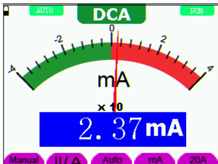
figure 24: DC Current Measurement for 400 mA
