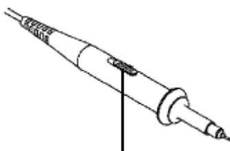
Figure 4-9 Attenuation Switch
