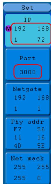
Figure 6-4 Set the network parameters of the oscilloscope
