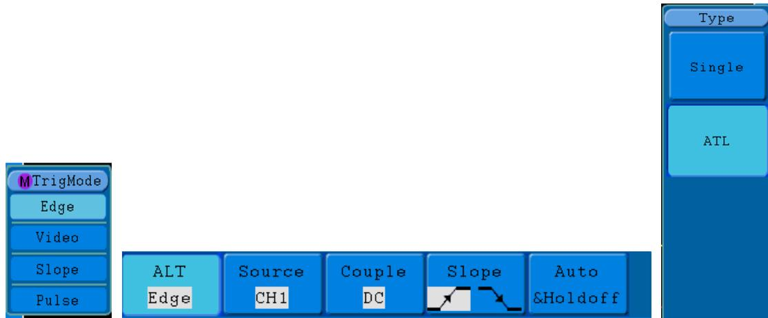
Figure 5-21 Alternate trigger (Trigger Type: Edge) Menu
