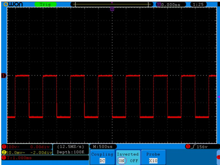
Figure 5-5 Inverted Waveform
