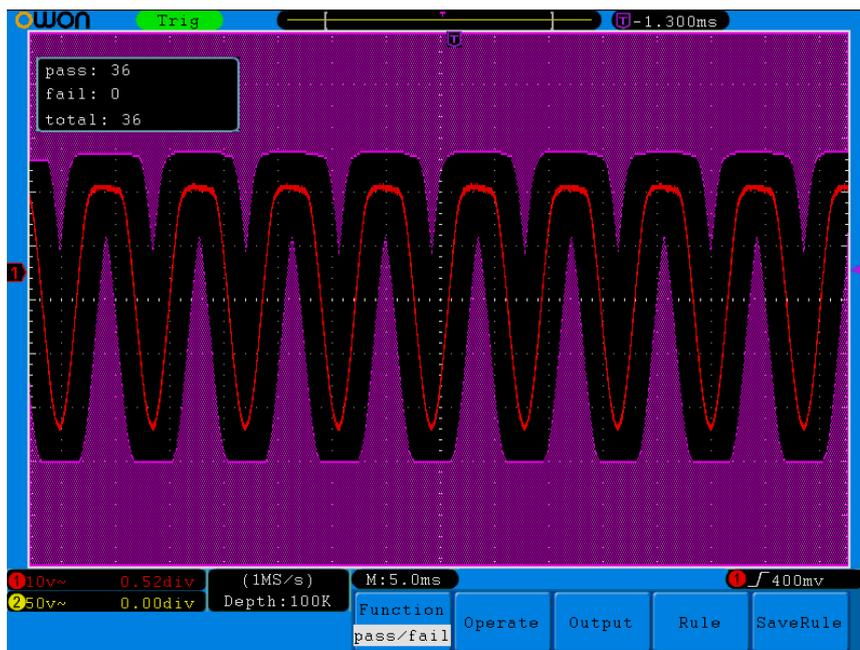
Figure 5-45 Pass/Fail test
