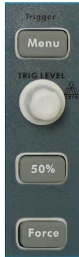
Figure 4-13 Trigger Control Zone
